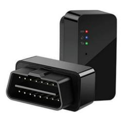
The Trova OBD is an easy-to-install plug & play OBD port tracker. With excellent location, tracking, reporting, logging, and security capabilities. The compact Trova OBD utilizes the GSM and GPRS communication networks along with GPS technology. This makes it an ideal solution for leased vehicles or large fleets.
